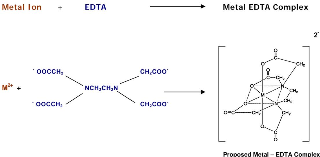
Metal chelates form over a broad range of pH and are highly soluble and extremely **stable**. Figure 2 below shows stability constants\*, K, of some metal chelates, expressed in logarithmic values. These values are indicators of stability of metal chelates; the higher the value the more stable the metal chelate and the harder it is to break and remove the metal.
